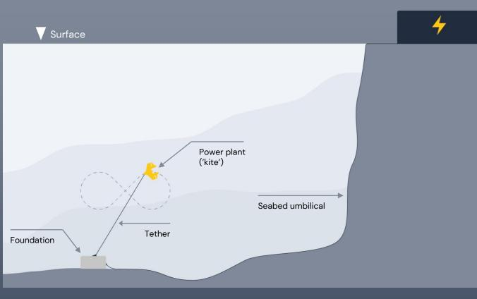
Wing creates lift force – pulls the turbine through the water
